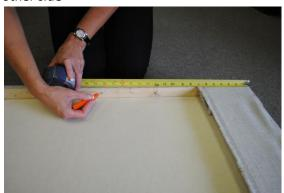
2. Place 1 bracket with the rear edge touching the cloth on the rear of the panel. Align the top of the bracket (wide slot faces the bottom of the bracket).
